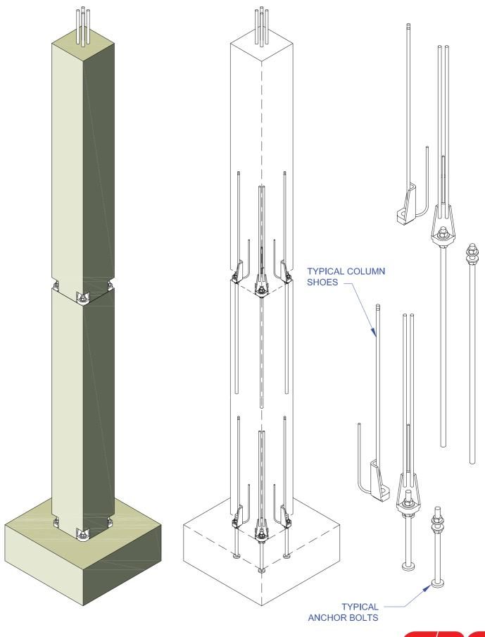
SIZE OF COLUMN SHOES AND ANCHOR BOLTS AS PER DESIGN REQUIREMENTS
